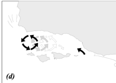
Figure 1. Different characteristic patterns of the surface circulation in the Santa Barbara Channel, derived by subjective review of 900 daily maps of average currents. These patterns account for the circulation over 60% of the time.
