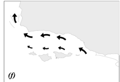
Figure 1. Different characteristic patterns of the surface circulation in the Santa Barbara Channel, derived by subjective review of 900 daily maps of average currents. These patterns account for the circulation over 60% of the time.
